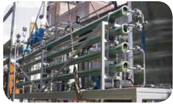
Brine recovery with nanofiltration
