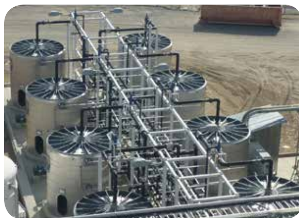
Separation of an organic acid with a chromatographic process
